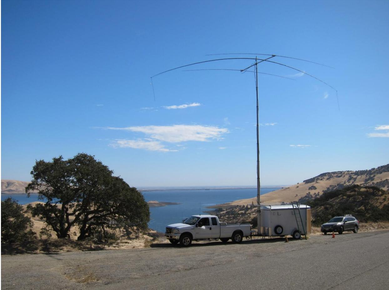
*Figure 4.* CQP 2019: KU6W antennas: 2-el 20m Yagi, 40m Dipole used on 15m&40m. Antennas at about 40-45ft.
