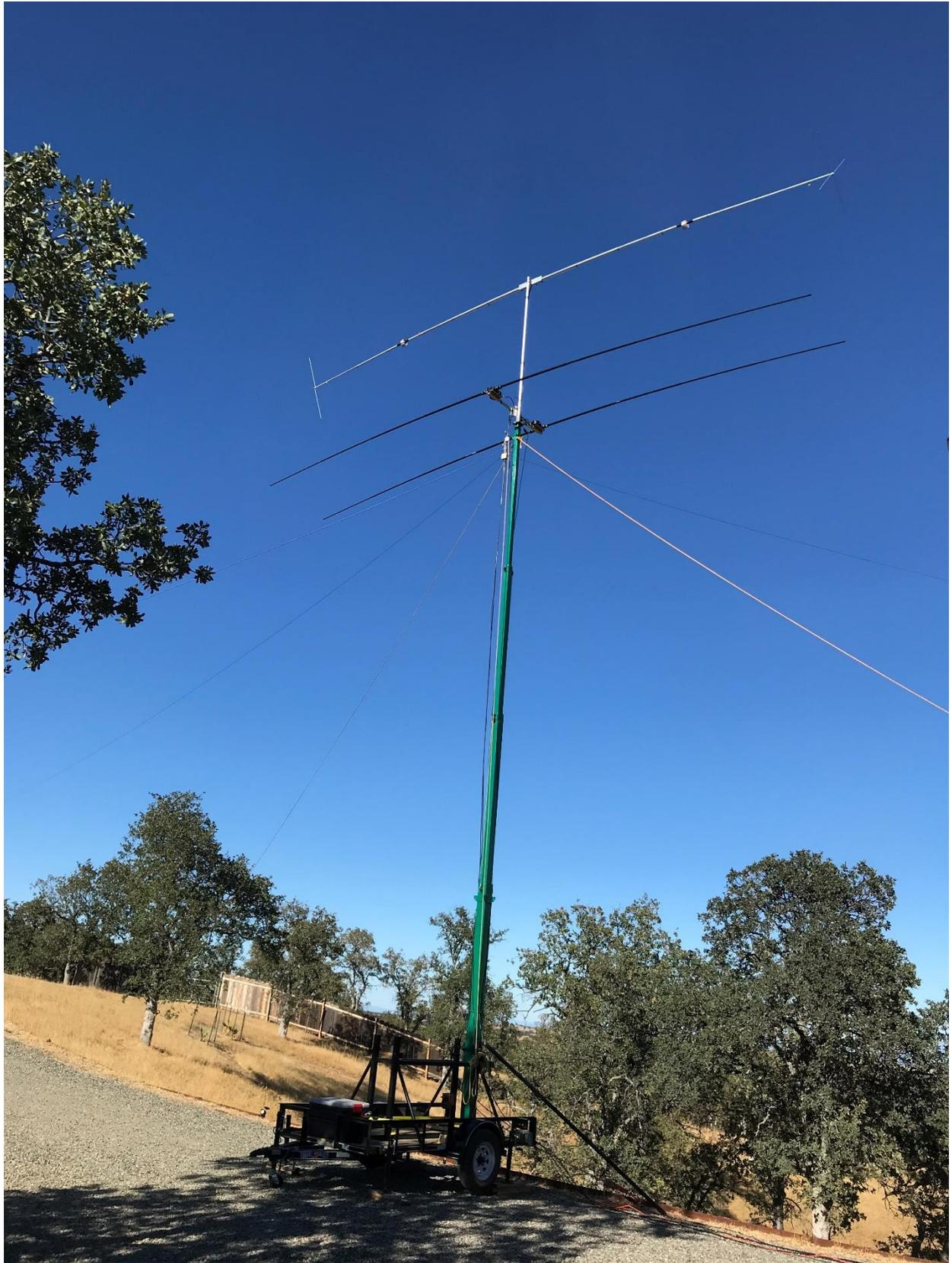
*Figure 6. CQP 2019: K6T antennas: 2-el SteppIR at 40ft, 40m Dipole at 50ft, 80m CW Inv-Vee at 37ft.*
